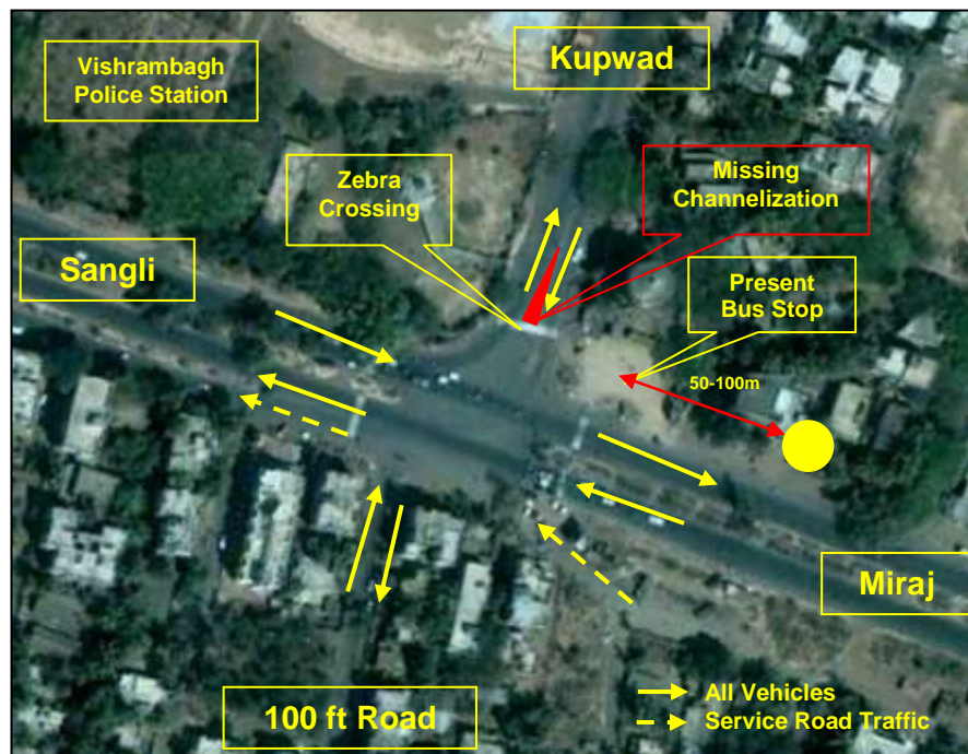
Figure 5-18 Vishrambagh Junction (At Police Head Quarters)
